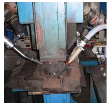
▲ FIGURE 3 In addition to the torch and interface, a torch cleaning device and a conventional GMAW power supply are shown.
