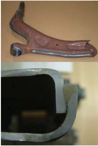
▲ FIGURE 4 This automotive control arm was welded with the hybrid process. A typical weld cross section is shown.
