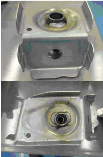
▲ FIGURE 5 A stamping and a tube are joined with two plasma/GMAW weldments.
