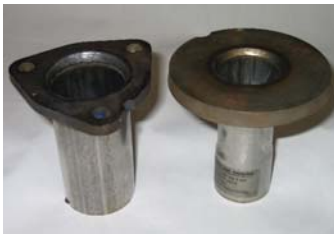
▲ FIGURE 10 Research has suggested that the quality and cleanness of plasma/GMAW welds are comparable with GTAW or plasma arc welds.
