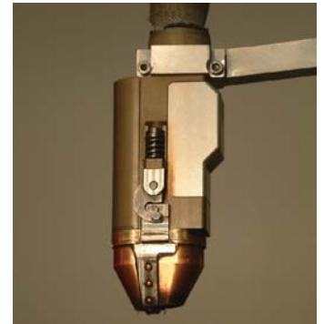
▲ FIGURE 2 This GMAW torch designed for the hybrid welding approach appears with the gas shield nozzle removed.
