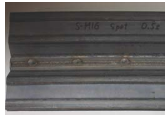
▲ FIGURE 7 This automotive bumper reinforcement was spot welded using the plasma/GMAW process.
