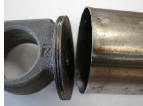
Parts for welding: Grooved mounting ring and tube to be welded
